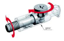
By turning the pinion screw, the threaded dowel makes a synchronized rotation.
