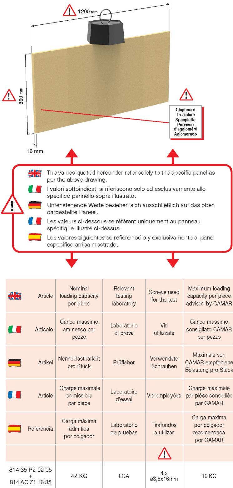
Any loading capacity advised here is the result of tests which refer to the panel as shown, correctly positioned and assembled, disregarding any construction variables of the finished panel, and disregarding the way it is fastened to the wall. We recommend that all dimensions which have been quoted in our technical drawings are complied with and **recommend testing a complete panel according to the norms which are in force in the countries where you intend to sell your products.**
