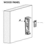
Recommended fixing countersunk screw type - head  $\emptyset$  4 mm max.
