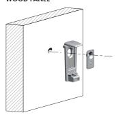
Recommended fixing countersunk screw type - head Ø 4 mm max.
