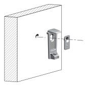
Recommended fixing countersunk screw type - head  $\varnothing$  4 mm max.
