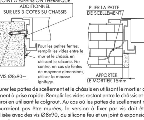
JOINT A EXPANSION THERMIQUE ADDITIONNEL SUR LES 3 COTES DU CHASSIS
