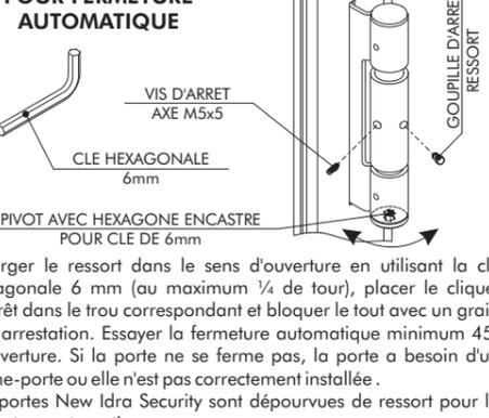
VIS D'ARRÊT AXE M5x5
