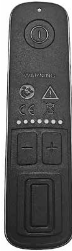
Start / Stop Tool starts / stops. Multi purpose led green. Speed indication active.
