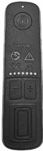
Warnings Multi purpose led red = over temperature Multi purpose led flashes green / red = voltage out of range
