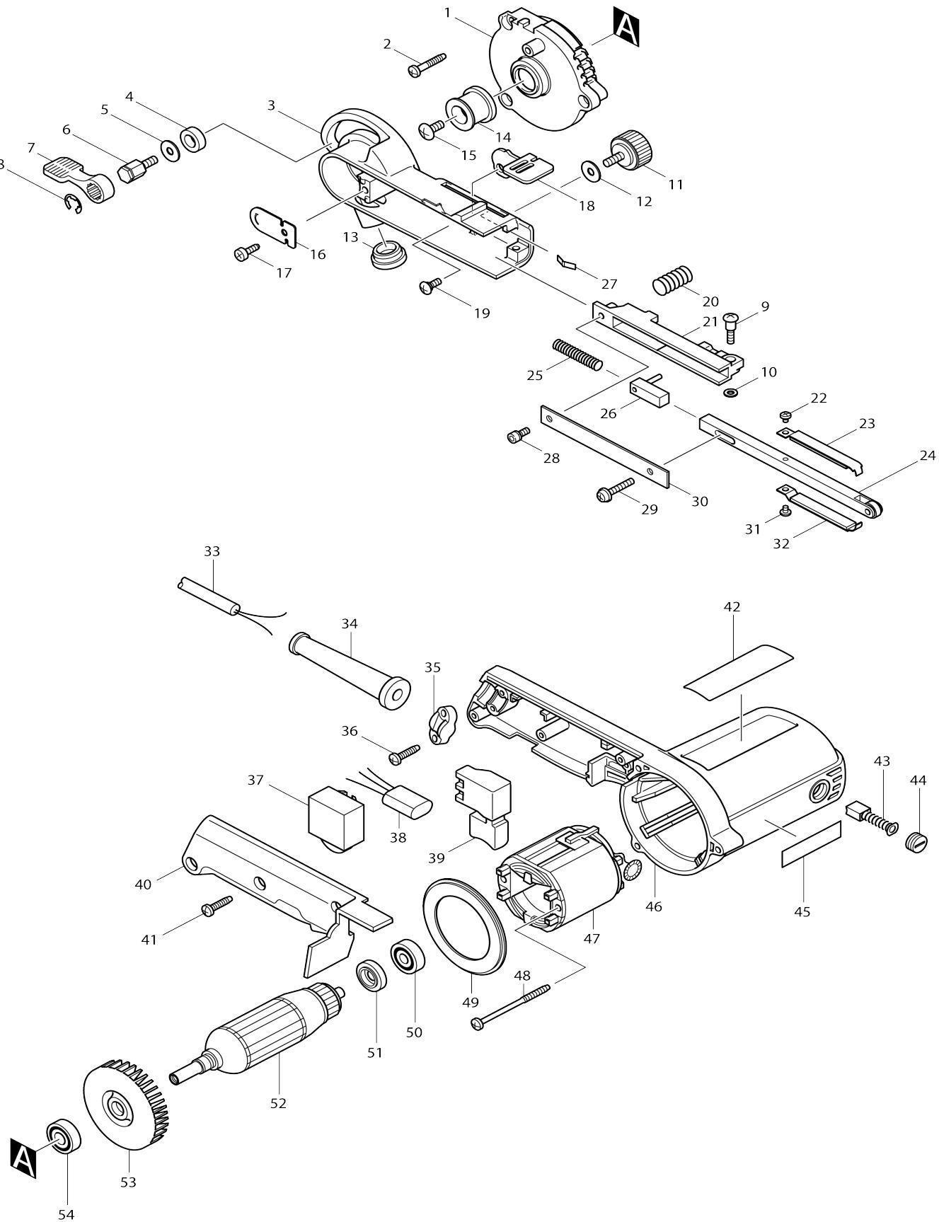
Model No.9032 PONCEUSE BANDE 500W D=9x533
