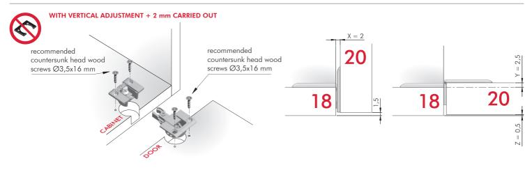
CABINET 19 mm WITHOUT ADAPTER - DOOR 16 mm WITH ADAPTER 2 mm THICK
